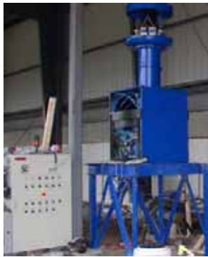
Figure 5. Field Installation of Pilot Squeeze Tower Press
